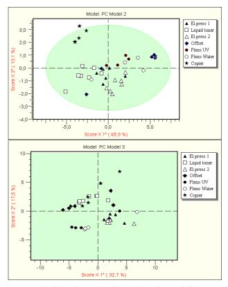
Figure 6: The multi variate data analyze show a difference between the different technologies in the data, the prints are grouped according to printing press in the score-plot The model based on perception attributes, top, and print quality measurements, bottom.
